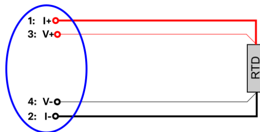
4-wire connection of a RTD probe to a circular connector
