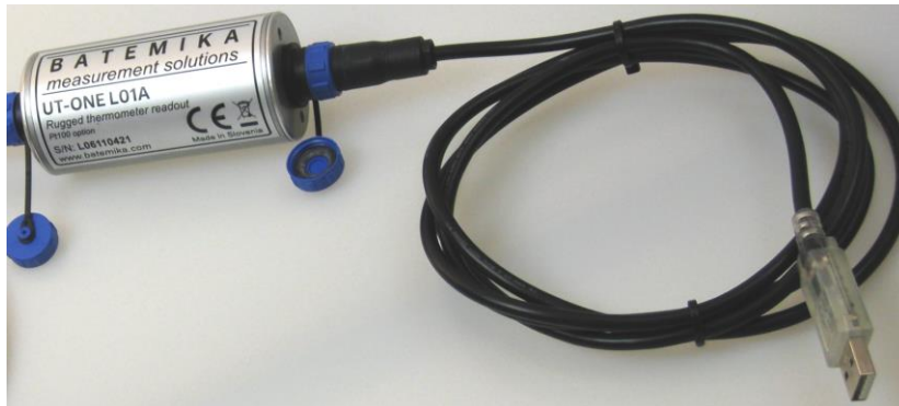
UT-ONE L01A with the provided USB to RS232 converter
